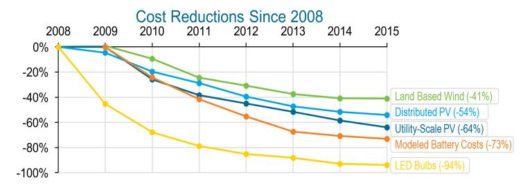
Notes: Land based wind costs are derived from levelized cost of energy from representative wind sites. Distributed PV cost is average residential installed cost. Utility-Scale PV cost is the median installed cost. Modeled battery costs are at high-volume production of battery systems, derived from DOE/UIS Advanced Battery Consortium PHEV Battery development projects. LED bulb costs are cost per lumen for A-type bulbs. See full report for full citations and details.
